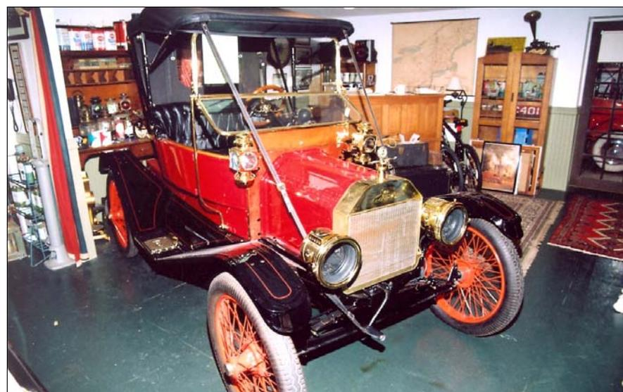
1911 T Torpedo with Rajo Head, Dual Winfield Carburetors
