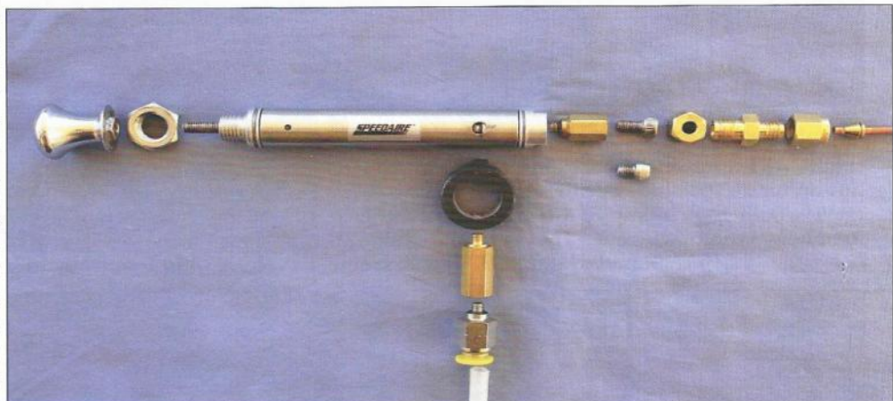
Exploded view of primer assembly with all components arranged in assembly position. Note extra 10-32 screw head ground to a taper for insertion within 3/16" compression fitting. View of completed primer assembly ready for installation in vehicle
