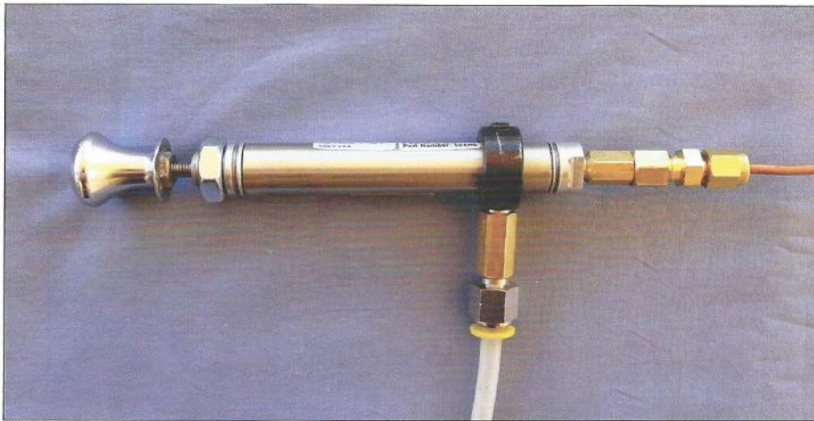
View of completed primer assembly ready for installation in vehicle
