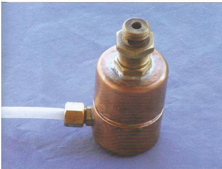
View of primer fuel chamber with top fitting soldered to chamber ready for assembling to fuel bowl in place of drain valve assembly. Side fitting is a 1/4" compression fitting soldered to chamber with nylon tubing directing fuel to primer assembly.
