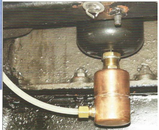
View of primer fuel chamber assembled to bottom of carburetor fuel bowl
