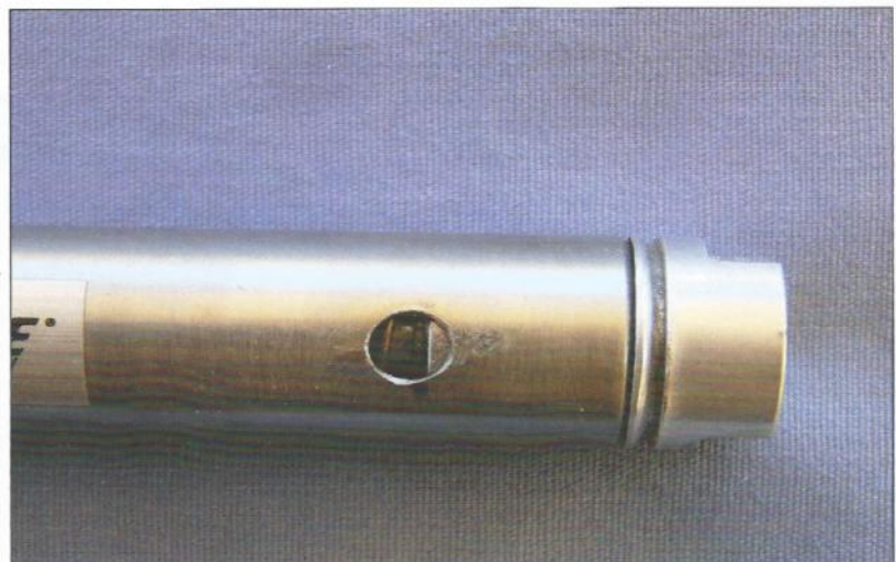
Close-up view of cylinder with 1/8" fuel inlet hole ground in cylinder wall
