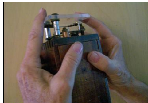
Using the Spring Gauge. A 4-40 pan head screw is used to indicate the two readings. Forty grams is indicated when the spring aligns with the top of the screw head, and 55 grams will align the spring with the bottom of the screw head. The spring element is made from an armature contact with the spring section ground down to a 1/8" width.
