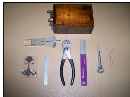
Using the Spring Gauge. A 4-40 pan head screw is used to indicate the two readings. Forty grams is indicated when the spring aligns with the top of the screw head, and 55 grams will align the spring with the bottom of the screw head. The spring element is made from an armature contact with the spring section ground down to a 1/8" width.
