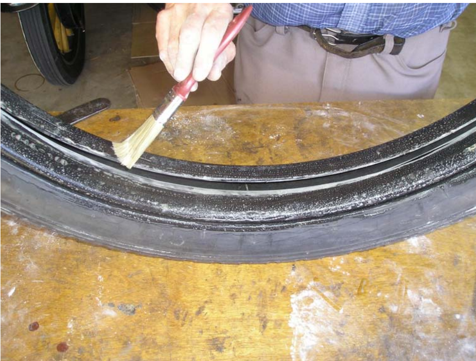
12. Coat the clincher bead with rubber lube.
