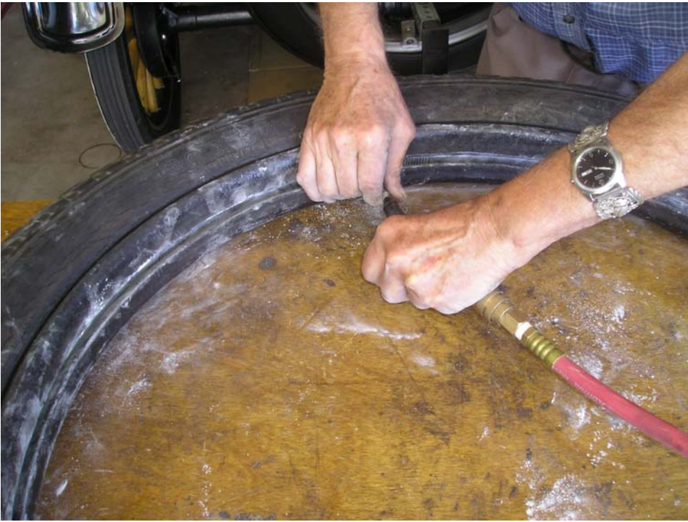
11. Inflate tube using rubber tipped air nozzle. Schrader valve removed.
