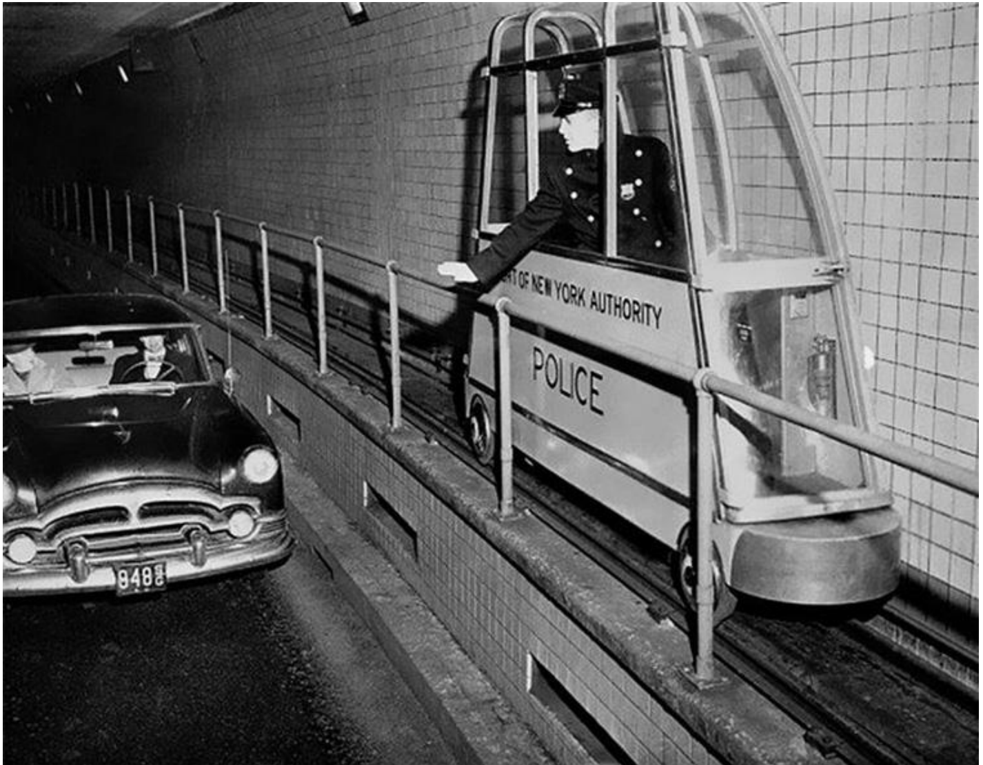
In 1955, This Tiny Electric Narrow Gauge Train Was Installed In New York's Holland Tunnel To Monitor Traffic Speed
